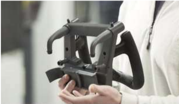
Fig. 6 Logo fixture 3D printed as single part for automotive assembly line[13].
