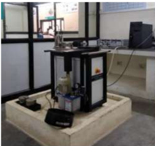
Fig 3. Pin on disk tribometer
