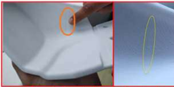
Fig. 8 Hairline crack developed after post-processing, caused due to high temperature gradient between part and soap solution
