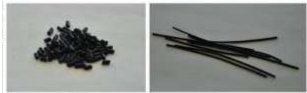
Figure 5 Graphene infused PLA pellets and 1.75 mm filaments.
