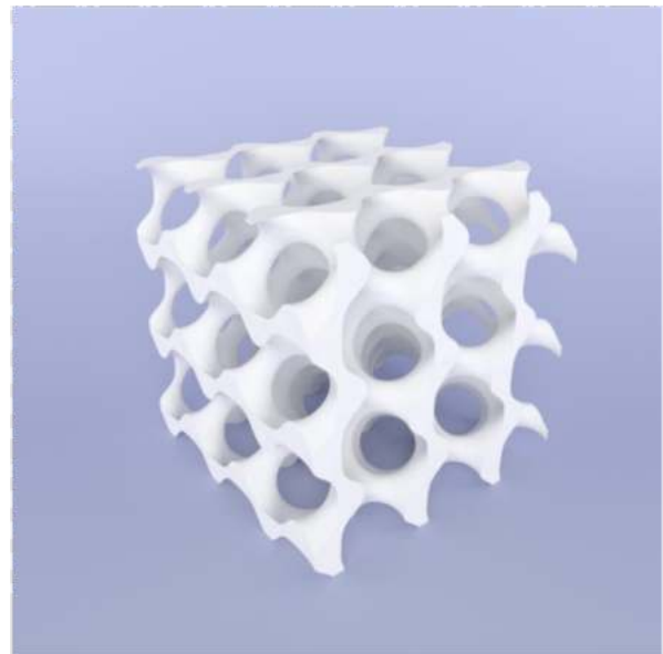
Fig. 1 Example of a Schoen Gyroid lattice structure
