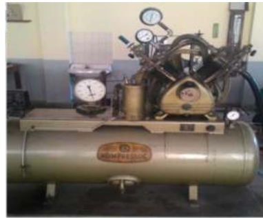
Fig 2.7: Multistage air-compressor in the Energy Conversion Engineering (ECE) Lab, BMSCE
