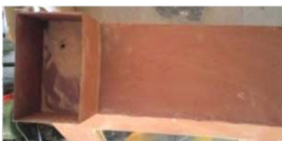
Fig3.4: Ceiling with abrasive reservoir compartment
